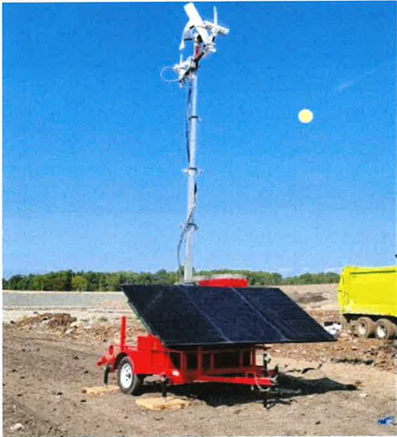
Landfill Fire Detection Unit
